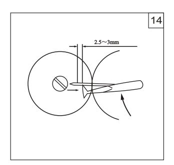
(c) The length between pinpoint of crochet hook and the center of needle eye should be  $2.5 \sim 3$ mm when pinpoint enters into the center of needle. (Fig 14) Loosen the screw to adjust.
