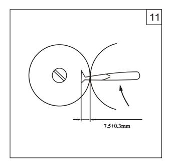
(6) Coordinate orientation between crochet hook and needle
